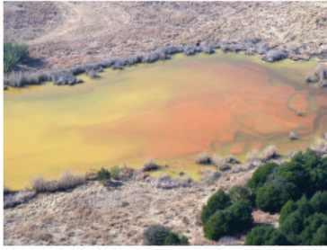
Hippo Dam, prior to the decant of AMD, known as the Dry Dam. Note the precipitated metals in the Dam.
