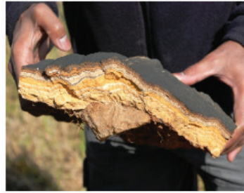
Metals in Acid Mine Drainage drops out as a precipitate after neutralisation or a pH adjustment (Photographs: Stephan du Toit)
