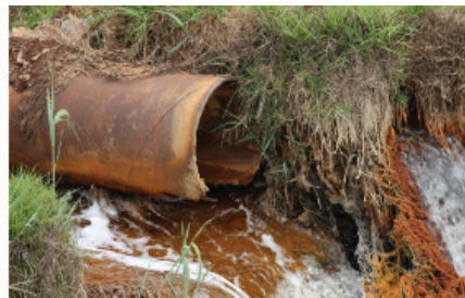
Pipes transporting Acid Mine Drainage. The first photograph shows a pipe with precipitated metals and the second photograph corrosion caused by acid mine drainage
