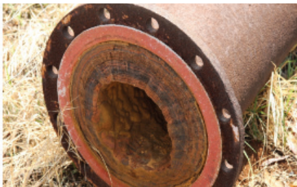
Pipes transporting Acid Mine Drainage. The first photograph shows a pipe with precipitated metals and the second photograph corrosion caused by acid mine drainage
